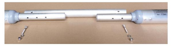
**DO NOT seal** the joints with adhesive tape or other similar element, the antenna MUST breathe otherwise you may have serious problems over time due to condensation or moisture. When the two seeds are ready, prepare the central plate and assemble all the parts as per photo. The two dipole ends must protrude from the insulator of 2.5cm and a spacing of at least 1cm
